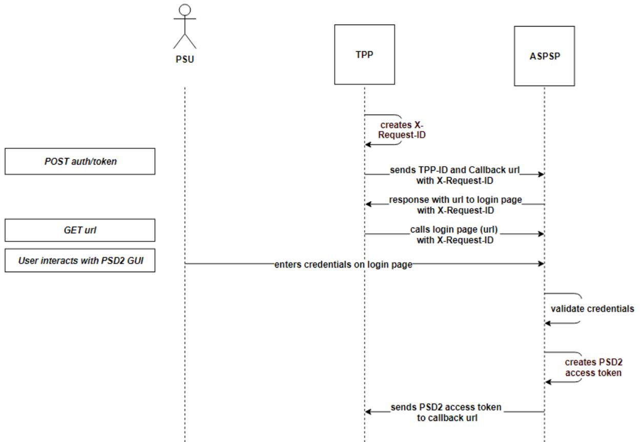
Figure 8 - Pre-auth Authorization code flow (SCA not necessary)
